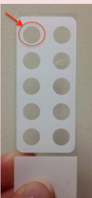
Fig. 4 – The microscope slide used to hold the water droplets. The drops were placed in the hole circled in red.
