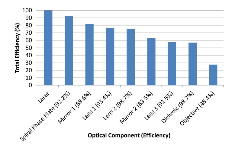
The percentage of power from the laser remaining after each listed optical component.
