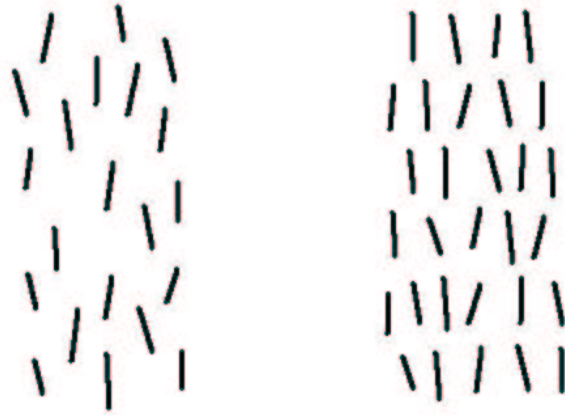
Figure 1: Nematic and smectic liquid crystal molecules, respectively, with orientational order. The director points upwards in both cases.
