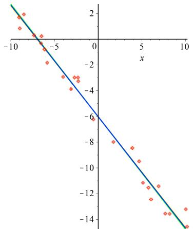
The differences between lsqx, lsqy and *mineuclid* are very small (as seen on the graph), but the best fit line to the curve (euclidian) would be used in replace of the standard least square method when very high accuracy is needed.
