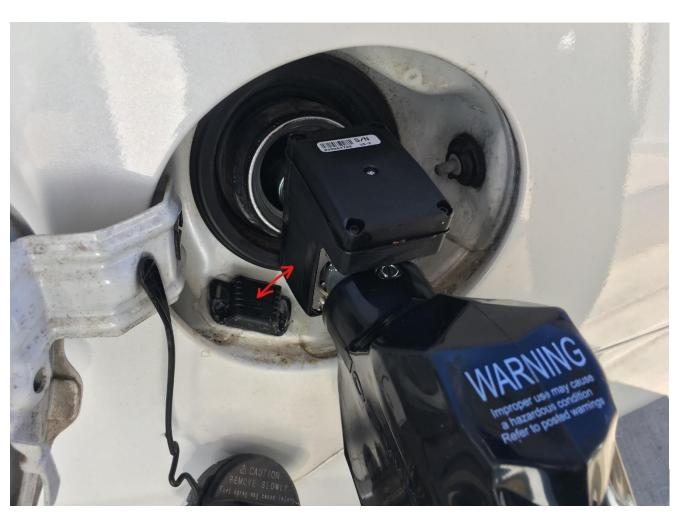
The nozzle must remain inserted all of the way in order to minimize the distance between the fuel cube or ring and the receiver. Once the nozzle is removed from the vehicle's filler neck or the distance between the receiver and transmitter becomes too great, the fuel pump will shut off.
