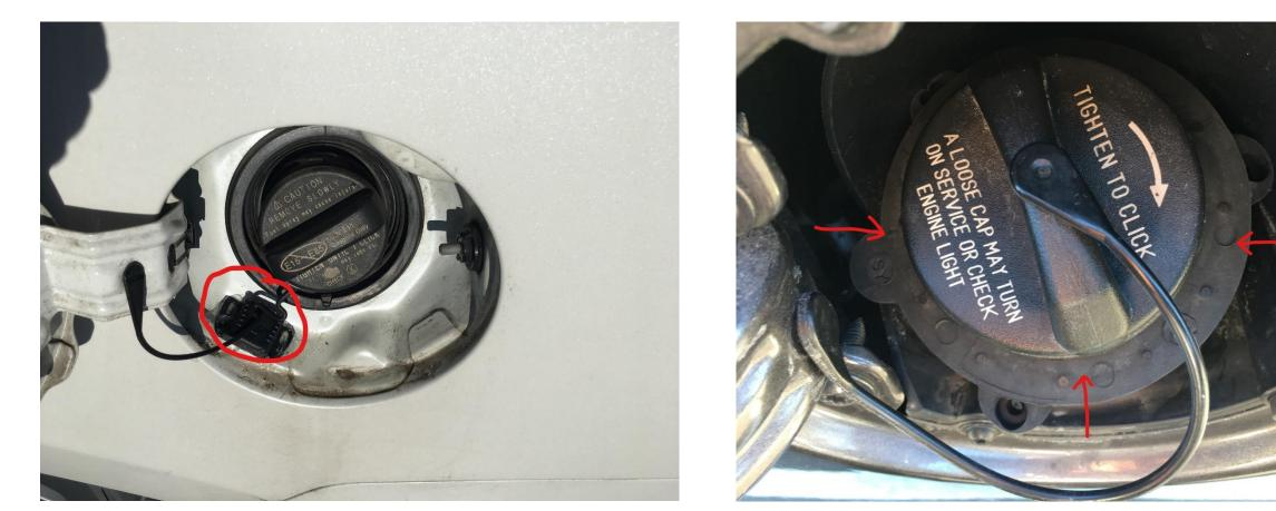
The fuel pump nozzle is equipped with a receiver that automatically recognizes the vehicle and allows fueling to take place.
