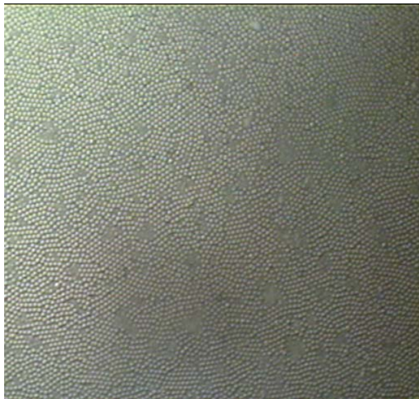
(a) Optical Microscope Image of 2 micron silica bead surface
