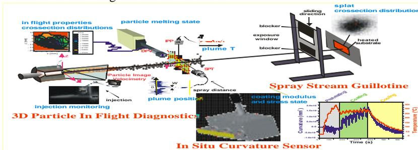
Fig. 1: Sensor set-up to explore process capabilities.
