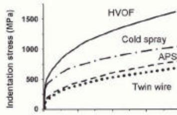
Fig. 1. Stress-strain curves for Ni-5%Al
