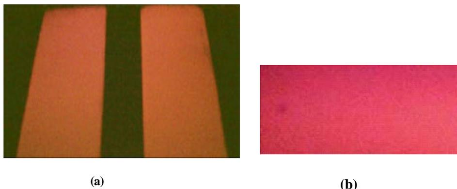
**Fig. 1: Red emission from (a) Eu-YAG and (b) Eu-Y<sub>2</sub>O<sub>3</sub> films when excited with a Mineralight UV lamp.**
