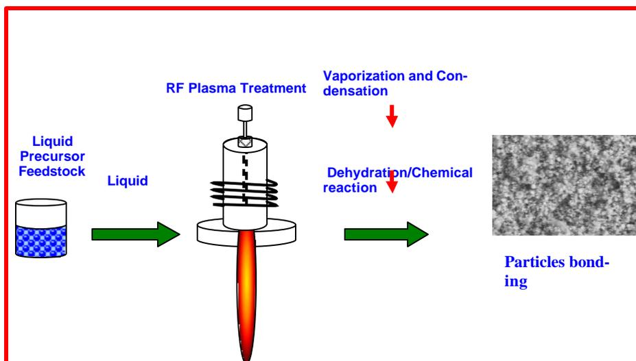
**Fig. 2: Schematic of precursor plasma spraying process.**
