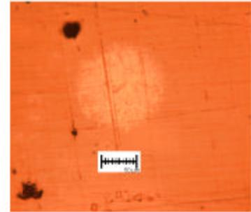
Fig. 2. Deposition of a porous Au film (40 nm thickness) allows determination of the contact diameter resulting from elastic indentation of the coating; all mechanical data can thus be generated from simple hardness testing.
