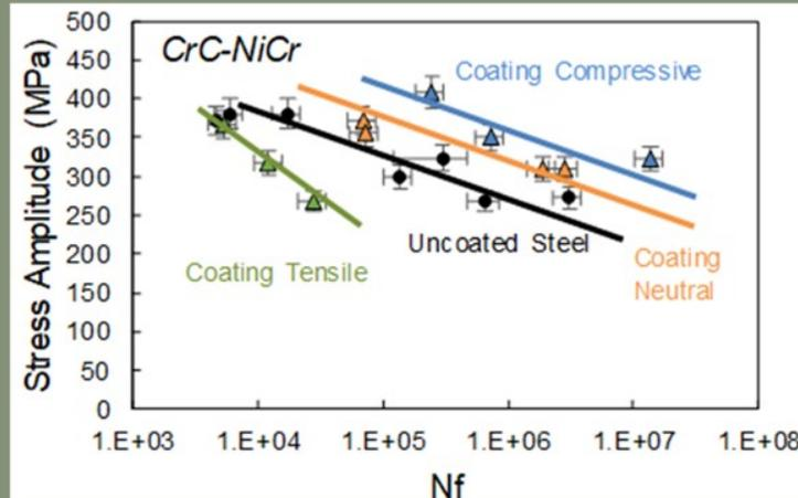
in the inset. As expected the compressive stress state sees a higher life (number of cycles, Nf) per stress amplitude as compared with the other coating states, and the uncoated steel substrates. The stress amplitude conversion compensates for the added material thickness. This assessment allows systematic analysis of coating modification, in the context of a highly repeatable and representative evaluation design.
