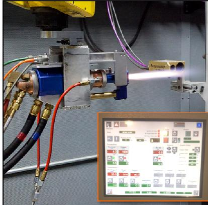
for a range of different materials and processes and incorporation of in situ and ex situ diagnostics for characterization of processes and resultant coatings.
