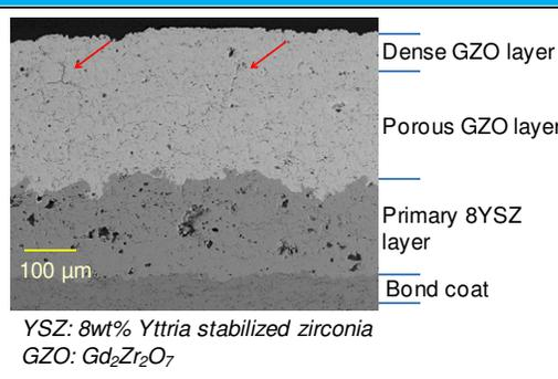
The figure also shows microstructure of one such fabricated multilayer sample. This particular sample matched or
