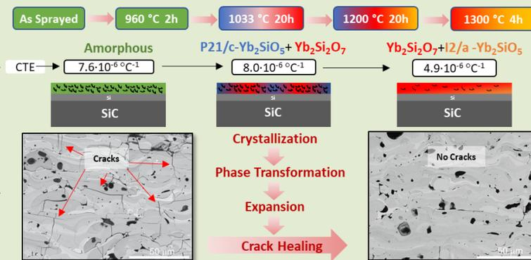
crystallization dynamics of the coatings and the importance of different silicate content. For instance, coatings with silica loss show the presence of the Ytterbium Monosilicate ( $\text{Yb}_2\text{SiO}_5$ ) phase during the crystallization and phase evolution process, leading to
