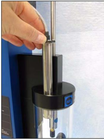
**figure 1-12.** *Insertion of Omega temperature/humidity sensor*
