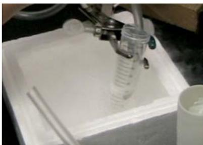
**figure 1-25. Condensing ethane in the conical tube**
