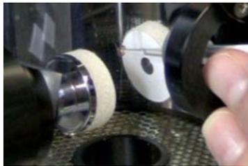
**figure 1-30. Applying sample aliquot to the support film**
