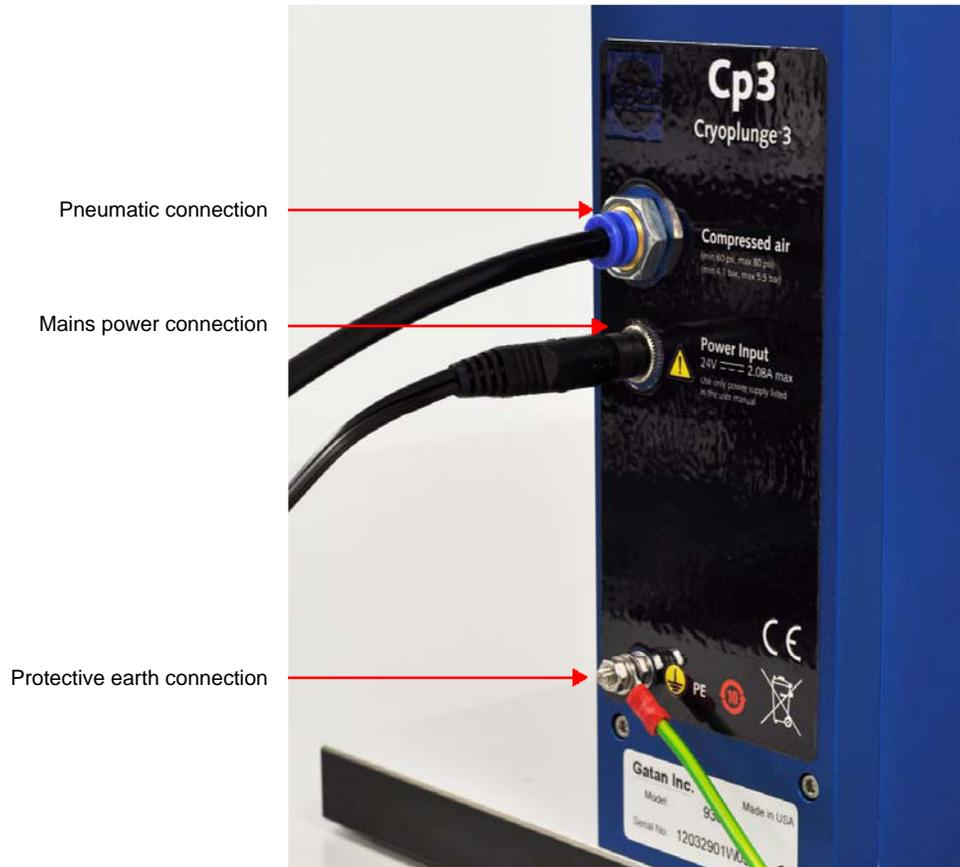
**figure 1-9. Pneumatic, mains, and protective earth connections**
