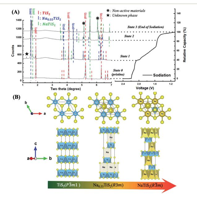
Fig. 5 (A) The *ex situ* XPD patterns from the TiS<sub>2</sub> electrode aligned with its corresponding electrochemical profile during sodiation. The peaks from non-active materials including the current collector are marked with (\*). (B) The major crystal structures involved in sodiation at each cycled state.<sup>39</sup>
