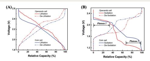
Fig. 2 The electrochemical profiles of the operando cell (red lines) as compared with the coin cell (blue lines) for lithiation/de-lithiation in (A) and sodiation/de-sodiation in (B).
