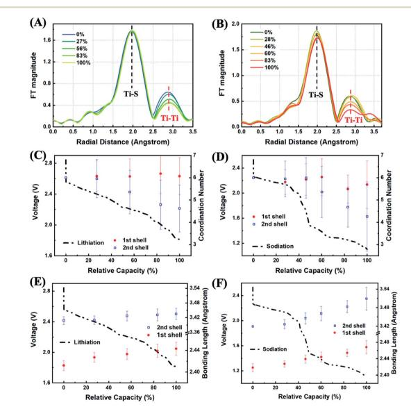
**Fig. 7** The radial distribution functions of the EXAFS part in *operando* XAS experiments during (A) lithiation and (B) sodiation at the various discharging states. The modeling results of EXAFS spectra on Ti-S (1<sup>st</sup> shell) and Ti-Ti (2<sup>nd</sup> shell): (C and D) Coordination number and (E and F) bonding length evolutions in both lithiation and sodiation.
