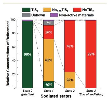
Fig. 6 The relative concentrations (%) calculated by Rietveld refinement at different discharging states as labeled in Fig. 5(A); the unknown phase is assumed to be  $Na_{0.3}TiS_2$  in the quantitative phase analysis.
