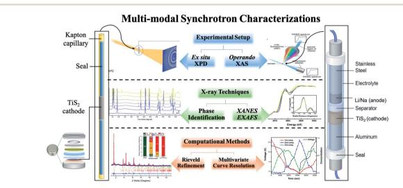
Fig. 1 Schematic of the multi-modal synchrotron characterizations for the *operando* and *ex situ* experiments at various beamlines and the corresponding techniques/analysis applied.
