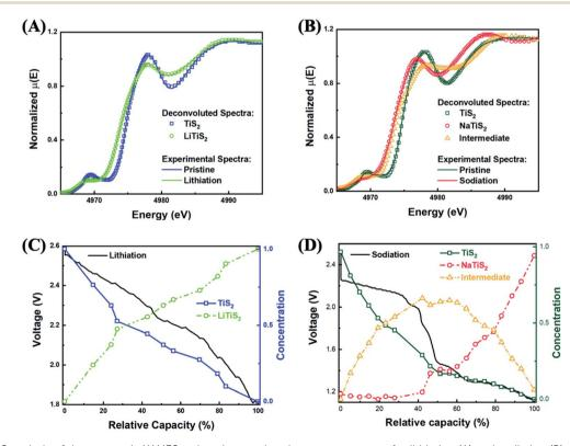
Fig. 4 MCR-ALS analysis of the *operando* XANES series: deconvoluted pure components for lithiation (A) and sodiation (B); the concentration evolution of two-component and three-component reactions for lithiation (C) and sodiation (D), respectively.
