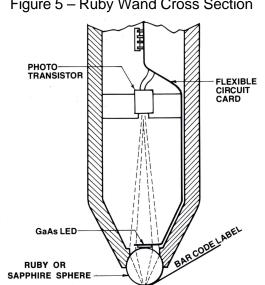
Figure 5 – Ruby Wand Cross Section
